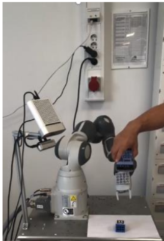
Figure 5: Lead-through programming of single-arm YuMi robot using 5G smartphone
