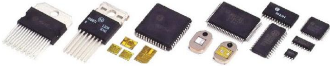
Figure 86: Examples of semiconductor packages (input to final test unit)
