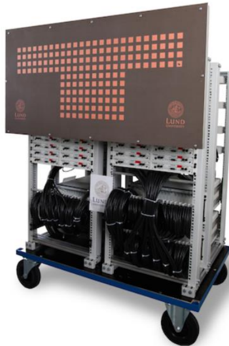
Figure 2: The Lund university massive MIMO (LuMaMi) testbed.
