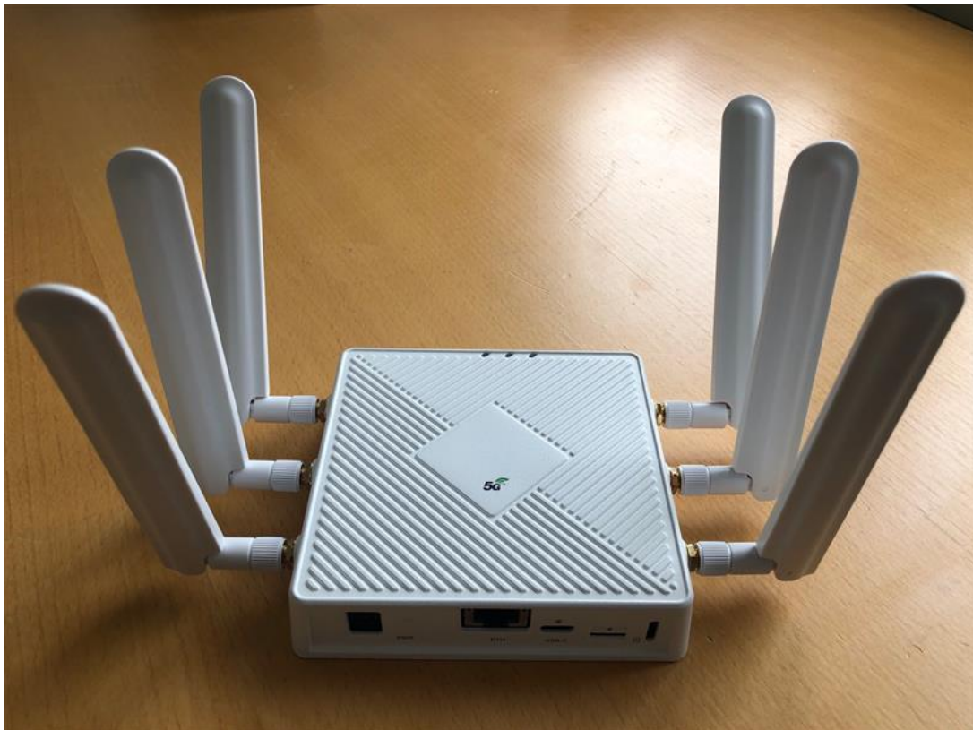
Figure 7 WNC Industry Router as a 5G UE used in the initial characterization of the acoustic emission monitoring use-case and 5G system performance evaluation
