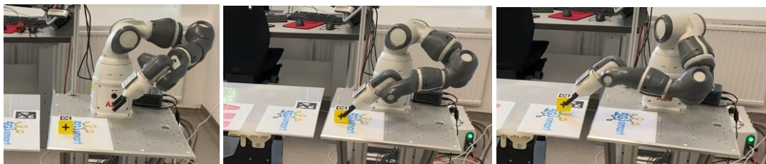
Figure 21 Execution service for the drop action, (a) home pose, cube pose estimated, (b) cube picked from the workstation, (c) cube dropped onto the mobile robot platform
