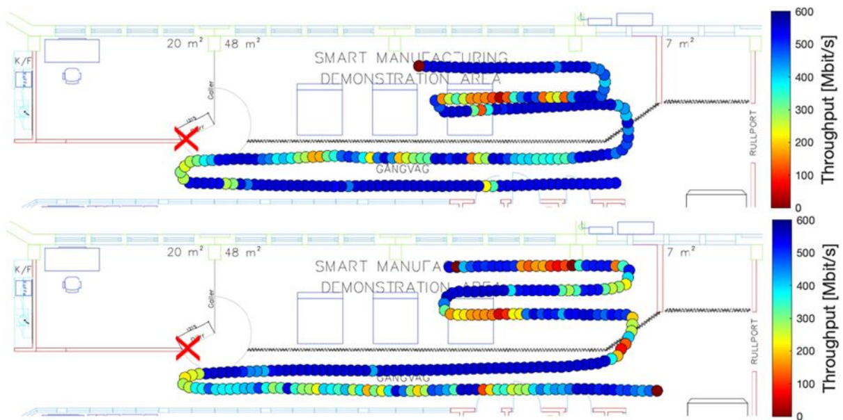
Figure 9 Coverage heatmaps over the test area, illustrated by DL throughput performance with UE B. In this case, throughput performance is substantially dependent on UE orientation. The red cross indicates the location of the base station antenna.
