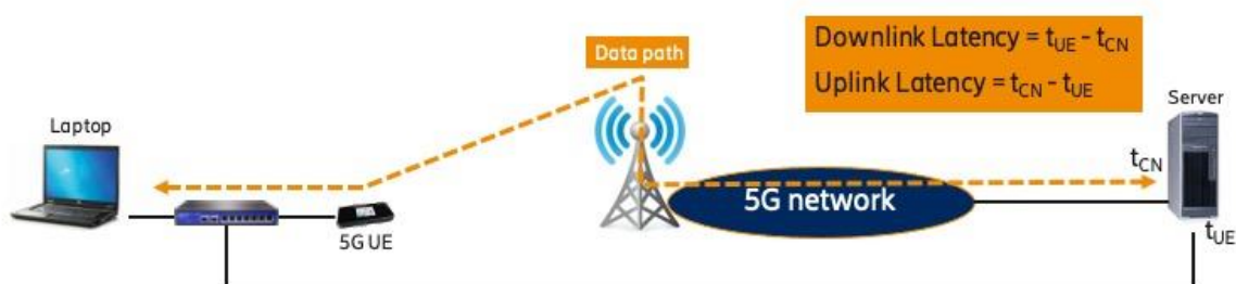
Figure 7 Latency characteristics network diagram
