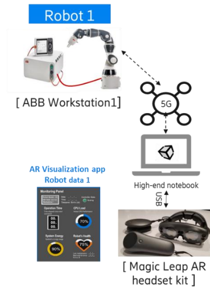
Figure 23 Test set-up for the validation scenario 1
