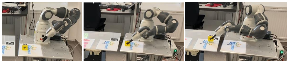
Figure 18 Execution service for the drop action on the cube, from left to right: (a) home position, cube's pose estimated, (b) the cube picked from the workstation, (c) cube dropped onto the mobile robot platform (source: ABB)
